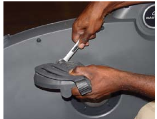
Figure 7 - Loosen left pedal nut
