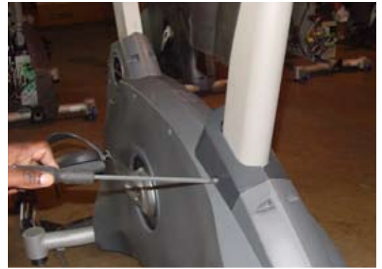
Figure 3a - Remove right mast cover
