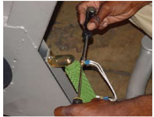
Figure 9a - Detach resistor wires (U916)
