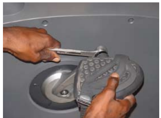
Figure 8 - Loosen right pedal nut
