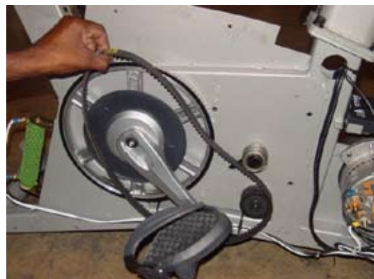
Figure 30 - Replace HTD Belt
