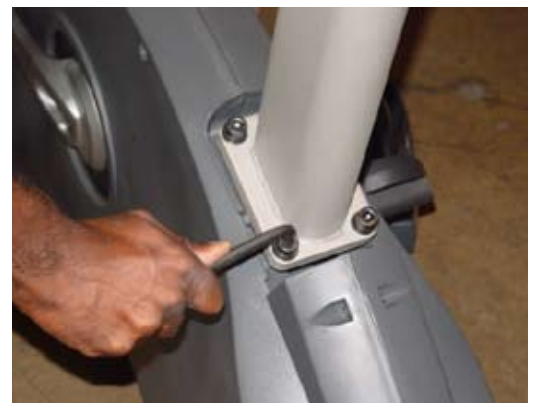
Figure 5a - Unbolt mast from frame (U916)
