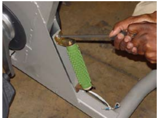
Figure 10a - Unscrew resistor (U916 shown)
