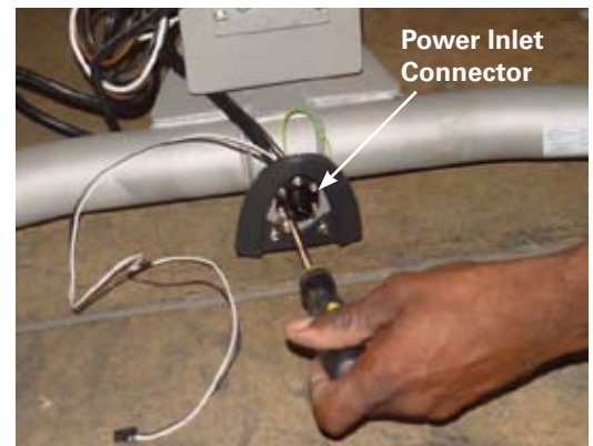
Figure 19a - Remove mounting screws
