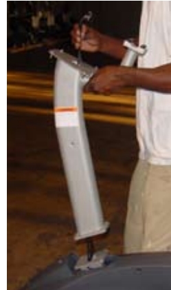
Figure 6a - Lift mast off frame (U916)
