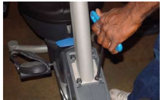
Figure 5b - Unbolt mast from frame (R916)
